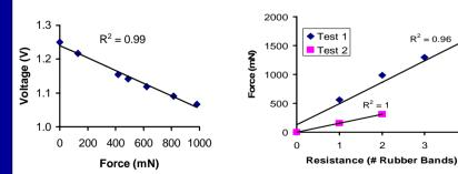
Calibration Curve. Calibration resulted in standard curve. Load cell test vielded a consistent linear relationship between force and voltage.
